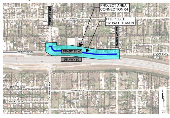
Connection 04 consists of the installation of approximately 1,650 LF of 16" HDPE main by open-cut along Brady Blvd. (TxDOT ROW) from Cupples Rd. to Barclay Rd.
